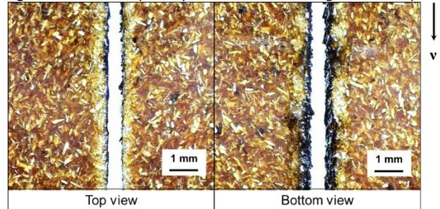
**Figure 7** Microscopic view of the laser cut for WPC at A1 – B1 – C1
