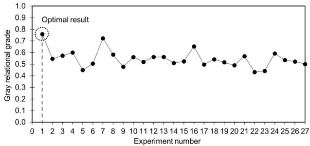
**Figure 5** Grey relational grade for multi-response optimization of single-mode pulsed fiber laser cutting of WPC
