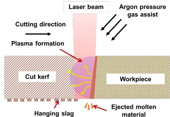
**Figure 2** Schematic illustration of fusion cutting of WPC
