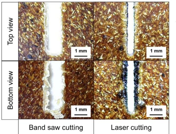
**Figure 1** The comparison between band saw cutting and laser cutting of WPC
