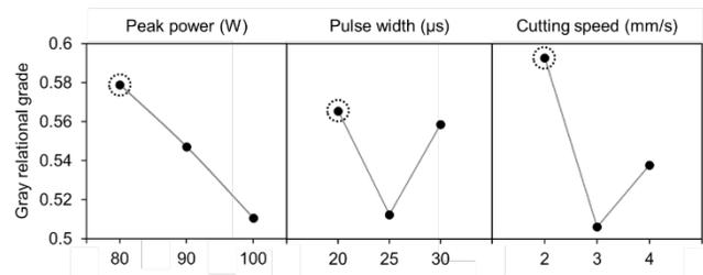
**Figure 6** Main effects plot of pulsed fiber laser cutting on multi-response
