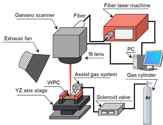
**Figure 3** Schematic diagram of laser cutting of WPC
