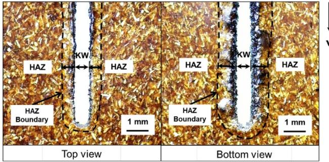
**Figure 4** The optical micrograph of measuring KW and HAZ
