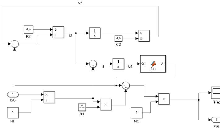
**Fig. 10. Subsystem simulink for supercapacitor two branch model**
