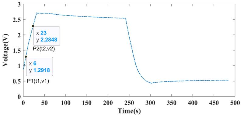
**Fig. 7. Experimental terminal voltage data of supercapacitor**
