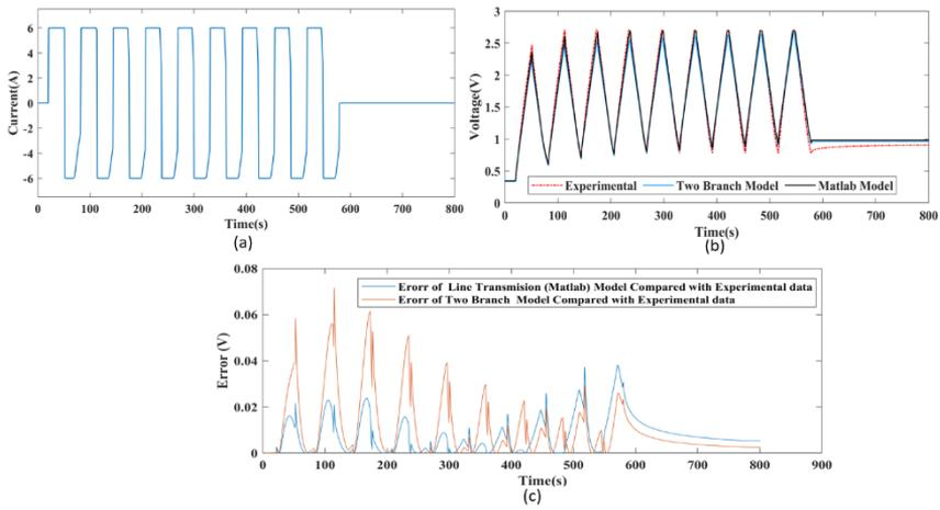
**Fig. 12. (a) Current profile (b) supercapacitor Experimental terminal voltage data, simulation two branch model and simulation of Line Transmission model (c) Error between measured and simulated models**
