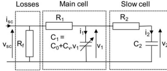
**Fig. 3. Supercapacitor two branches model [14]**
