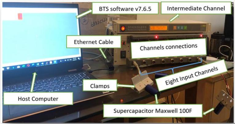
**Fig. 4. Experimental set-up**
