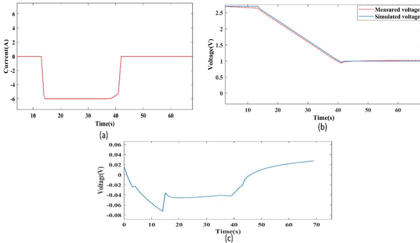
**Fig. 13. (a) Current profile (b) Rest-discharging terminal voltage validation (c) Error for rest and discharge validation of supercapacitor voltage**
