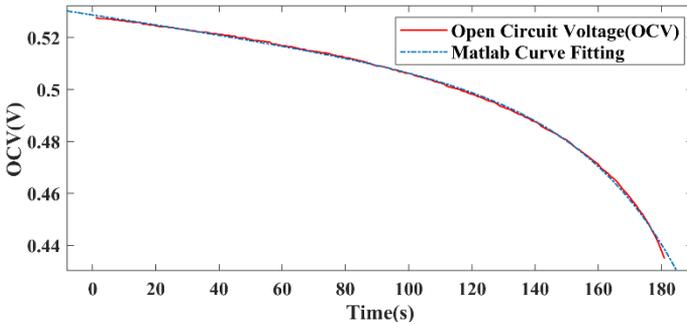
**Fig. 8. Terminal voltage during discharge curve**
