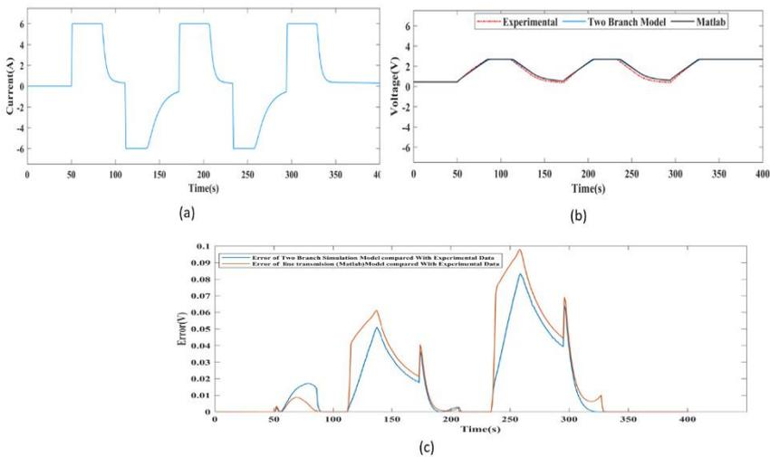
**Fig. 11. (a) Current profile (b) supercapacitor Experimental terminal voltage data, simulation two branch model and simulation of Line Transmission model (c) Error between measured and simulated models**
