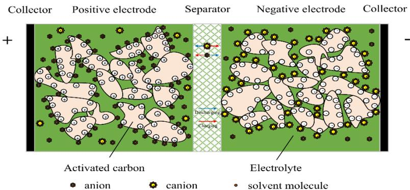
**Fig. 1. Supercapacitor cell structure**
