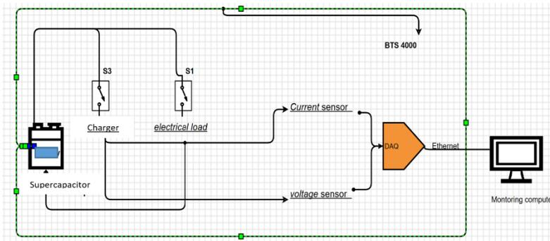
**Fig. 5. Neware battery testing system BTS4000**
