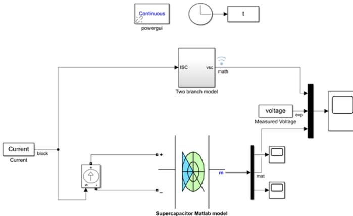
**Fig. 9. Matlab model and two branch model simulation**
