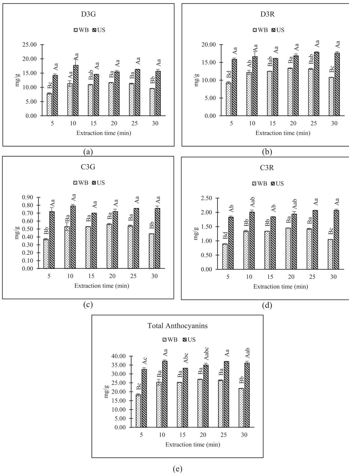
**Fig. 3.** Anthocyanin content in DBP extract during ultrasonication (US) and water bath (WB) extractions at different times, as measured by HPLC. D3G: Delphinidin-3-O-glucoside, D3R: Delphinidin-3-O-rutinoside, C3G: Cyanidin-3-O-glucoside, and C3R: Cyanidin-3-O-rutinoside. Values with different uppercase letters in each extraction time are significantly different ( $p < 0.05$ ). Values with different lowercase letters in each extraction method are significantly different ( $p < 0.05$ ).
