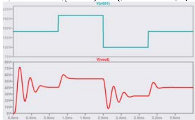
Figure 7. Unstable voltage output corresponding to stepping input voltage using LTSpice piecewise linear functions.
