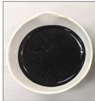
Figure 2. POFA based geopolymer using 10% POFA material
