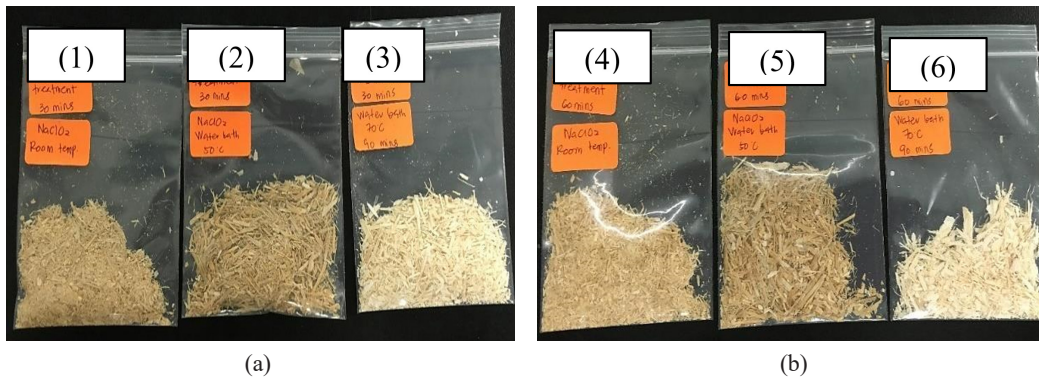
Figure 3. Physical appearance of fibre after steam and bleaching treatment; (a) steam treatment 30 min with bleaching treatment at (1) room temperature; (2) 50°C; (3) 70°C (b) steam treatment 60 min with bleaching treatment at (4) room temperature; (5) 50°C; (6) 70°C
