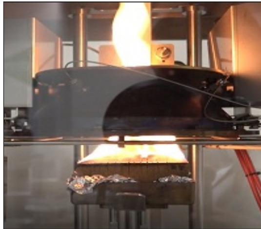
Figure 2. Timber surface radiated to get burned
