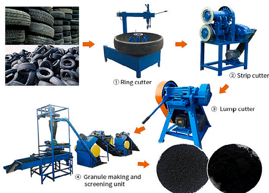
Fig. 1. Shredding of waste tire (Mhaya et al., 2021).
