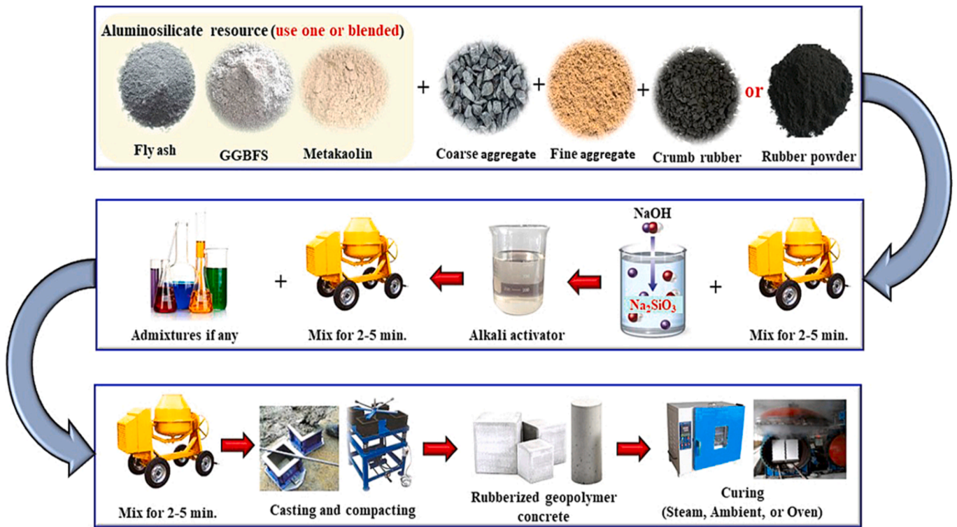
Fig. 5. Commonly used method of mixing RuGPC (Alawi Al-Sodani, 2022).
