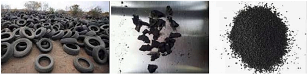
Fig. 1. (a): Waste, Fig. 1(b): chips, Fig. 1(c): Crumb rubber (Ali and Hasan, 2019).
