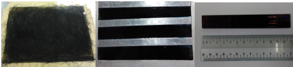
Figure 1. Moulding for: (a) Randomly distributed APREC; (b) Unidirectional APREC; and (c) standard size specimen after grinding process
