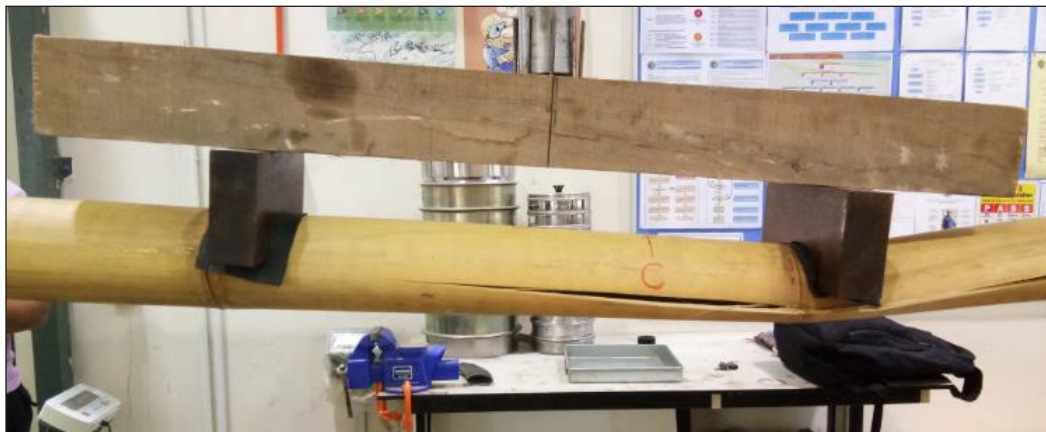
Figure 2. Local failure of bamboo due to crushing and splitting
