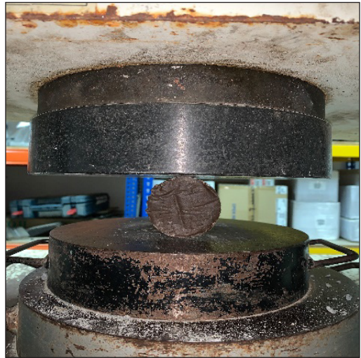
Figure 7. Splitting tensile test
