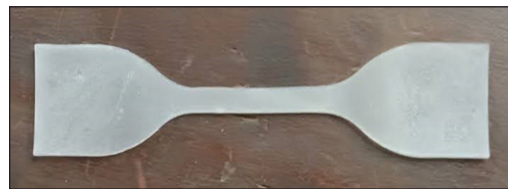
Figure 1. PDMS sample based on ASTM D412 type C standard
