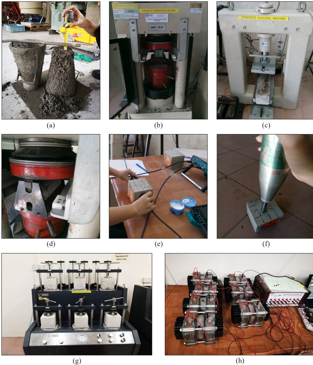
Figure 1. Test setup of (a) slump, (b) compressive strength, (c) flexural strength, (d) splitting tensile strength, (e) UPV, (f) rebound hammer, (g) water penetration, and (h) RCPT
