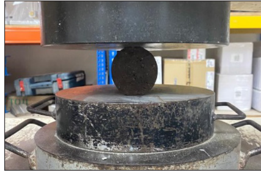
Figure 5. Lateral compression load of polymer concrete
