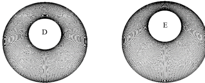
Figure 3 (Continue). Inner cylinder location and computational mesh for D: \epsilon = +0.333 ; E: \epsilon = +0.625
