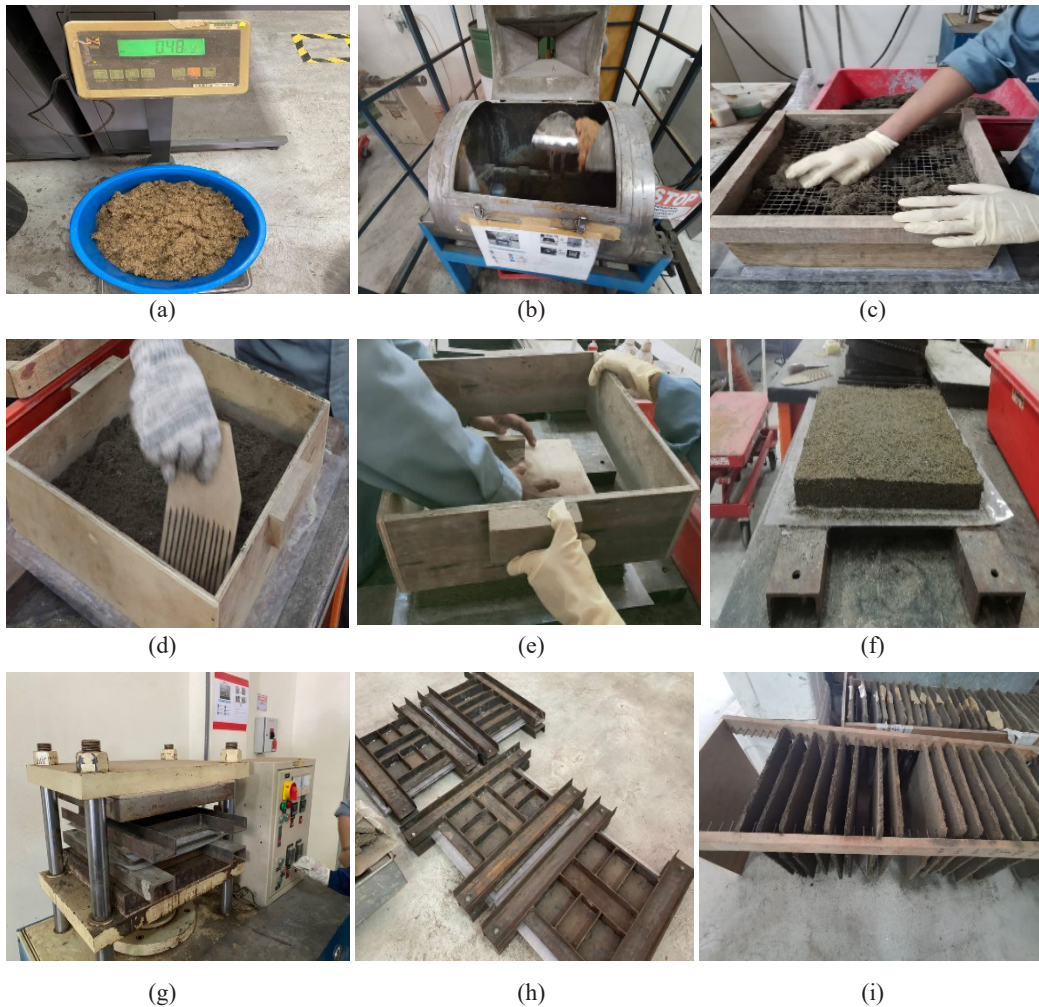
Figure 2. EFBCB fabrication process. (a) Weighting material, (b) Mixing process, (c) Spreading process, (d) Flattening process, (e) Pre-compact process, (f) Pre-forming process, (g) Compressed using compression machine, (h) Clamped process, (i) Curing process
