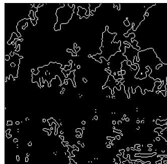
(f) Zero-cross-based edge detected image
