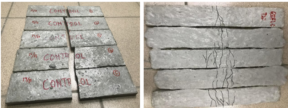
Figure 5. Failure modes under three-point bending test
