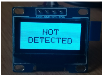
Figure 7. Default message for when error temperature is detected
