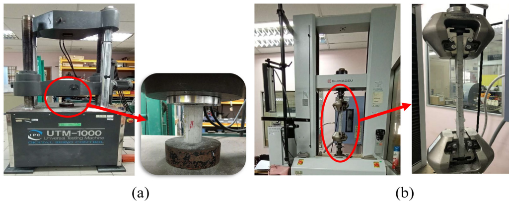
Figure 2. Testing set-up (a) uniaxial compression test and (b) uniaxial tensile test
