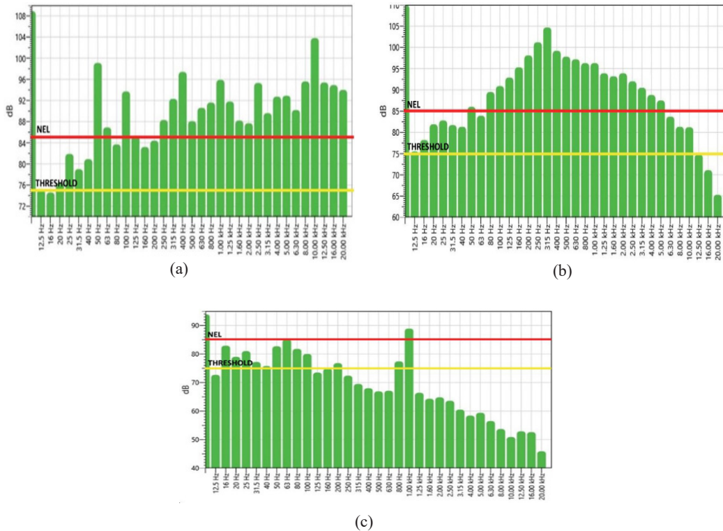
Figure 5. (a) Gas turbine A source reading; (b) Gas turbine A path reading; (c) Gas turbine A receiver reading
