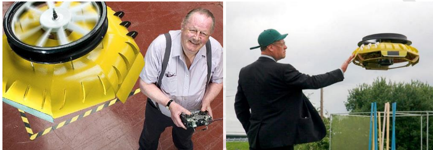
Figure 3: The Coanda UAV designed by Geoff Hatton (Hatton, 2010)
