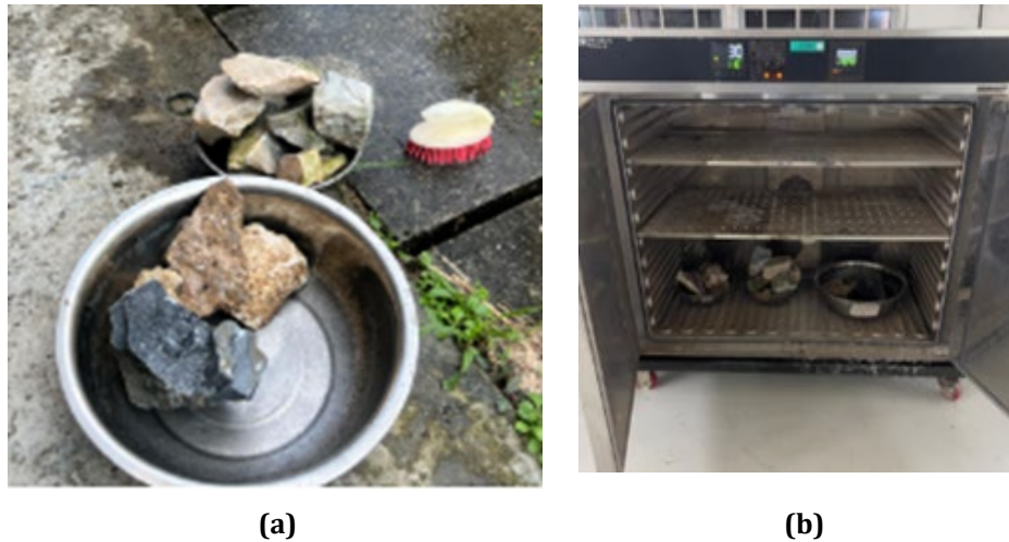
Fig. 2 Limestone samples in the laboratory for characteristic testing (a) washing; and (b) drying process
