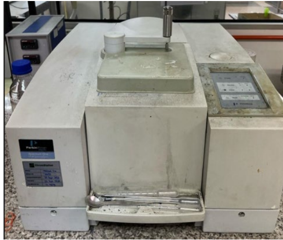
Fig. 4 Indicates the Fourier Transform Infrared Spectroscopy (FT-IR) analyser
