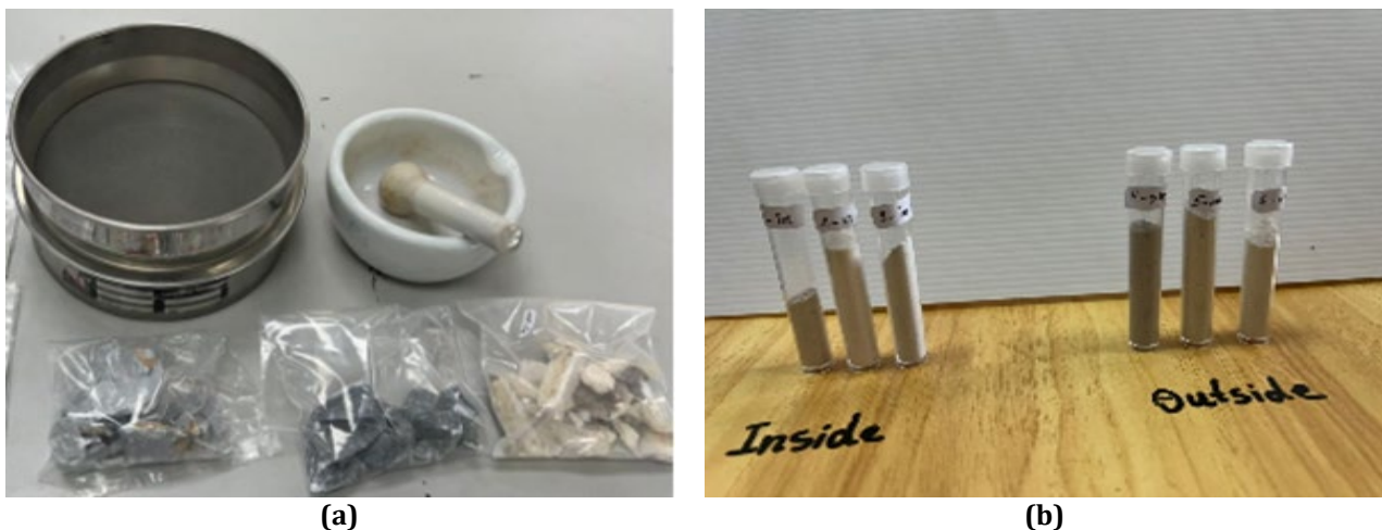
Fig. 3 Limestone sample preparing process (a) particle size reduction using appropriate tools - crushing and sieving of limestone samples; (b) labelled limestone samples for characteristic testing
