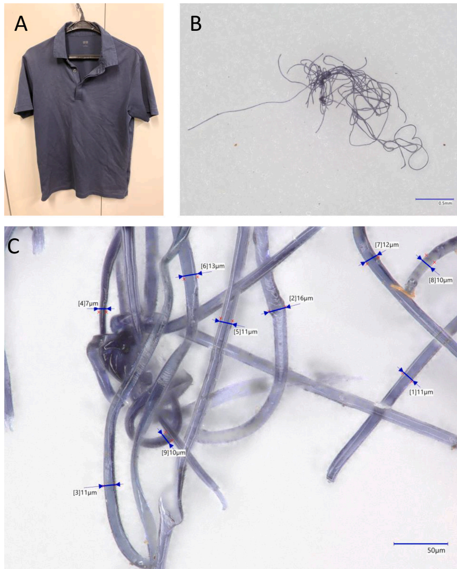
Fig. 1. Fibrous microplastic used in this study: a) pullover shirt from which fibrous microplastic was taken, b) fibrous microplastic taken from the shirts, and c) enlarged view of b), showing the thickness of the fibres.
