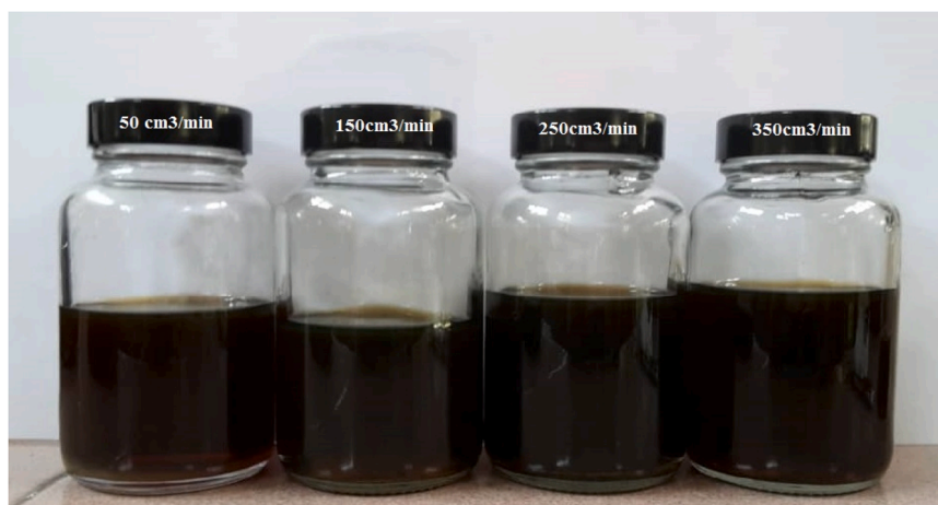
Fig. 6. The green diesel generated at different flows of nitrogen gas.
