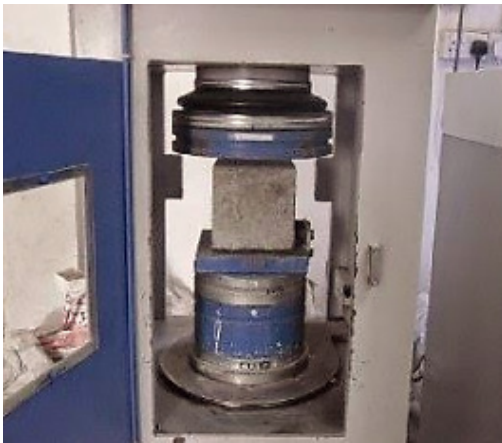
Figure 3. SCC cube under axially compressive loading
