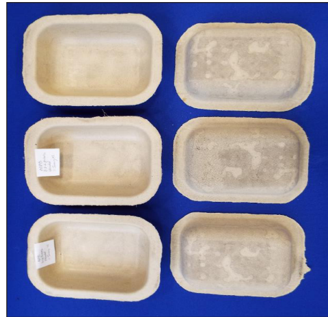
Figure 3. Punnets made from atmospherically refined EFB fibre
