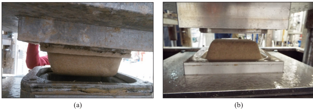
Figure 5. Current concave forming mould (a) and the new convex forming mould (b)
