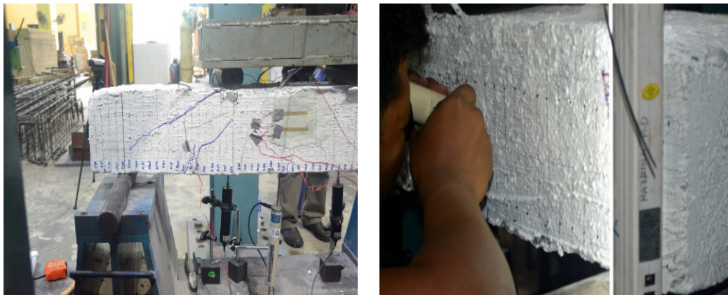
(b) Measurement of crack widths via optical magnification X10 microscope
