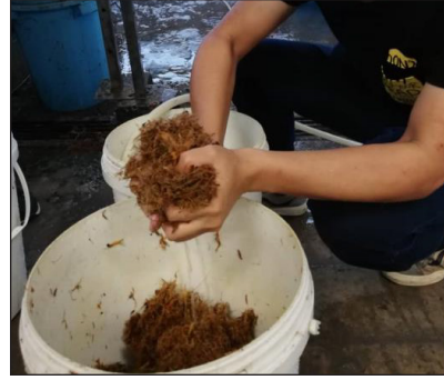
Figure 1. Fibres were properly washed to remove unwanted residue and debris
