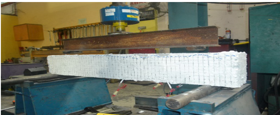
(b) Universal Testing Machine (UTM) was used to conduct the beam load test
