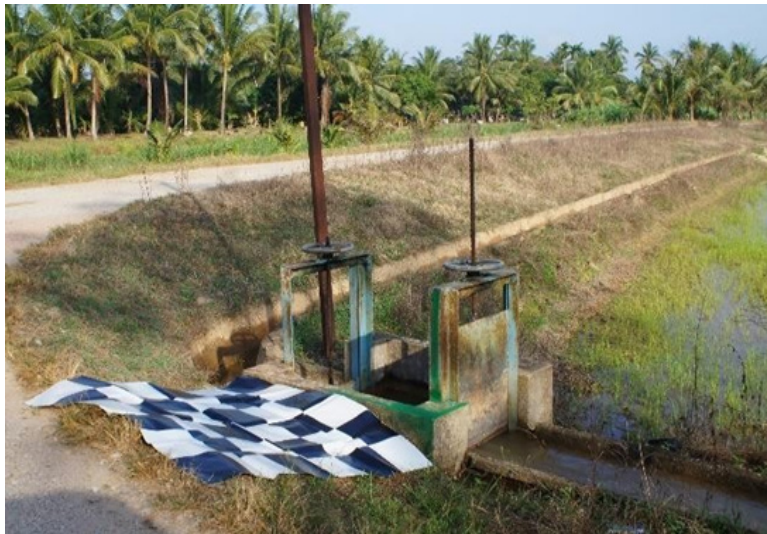
Figure 4. The GCP placed at the corner of the paddy field.
