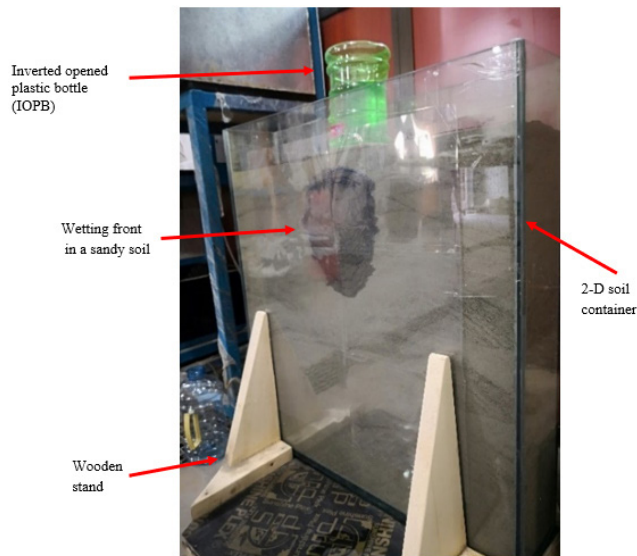
Figure 4. Experimental setup of the free-flow infiltration from the inverted open plastic bottle (IOPB)
