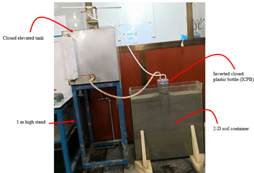
Figure 6. Experimental setup of bubble-flow infiltration from the inverted closed plastic bottle (ICPB)
