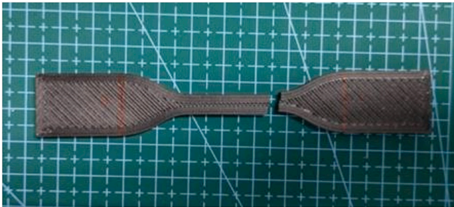
Fig. 10. Fractured location of the nonheat-treated sample.
