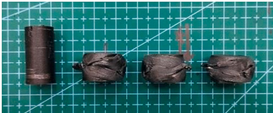
Fig. 15. Compressive sample before and after the test.
