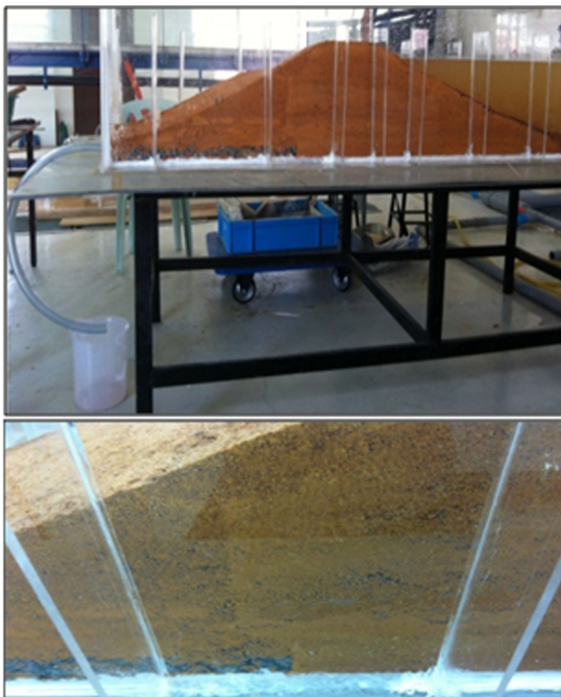
Fig. 6 Seepage line within the body of embankment models
