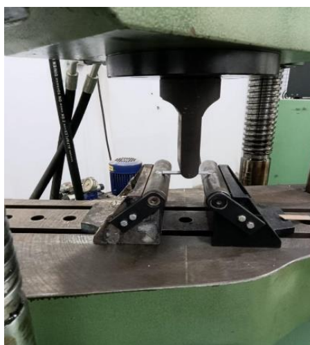
Figure 18: Flexural test (ASTM D790) of AgNP+PLA
