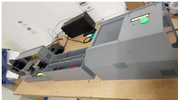
Figure 6: Filament extrusion setup
