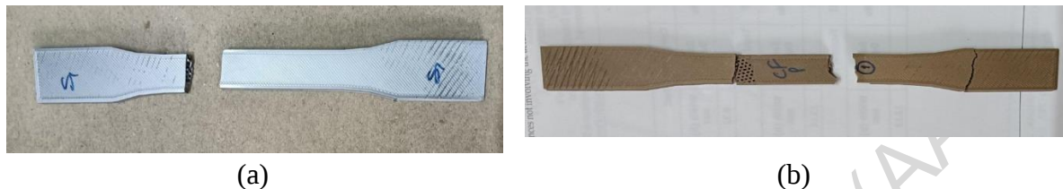
Figure 3: Tensile specimens (ASTM D638) (a) silver nanoparticle induced PLA (b) copper nanoparticle induced PLA
