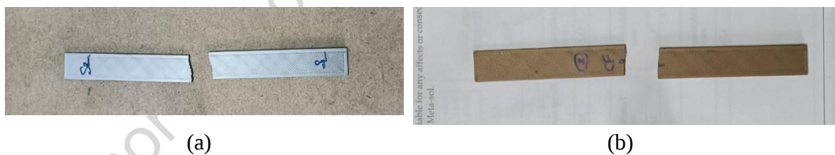
Figure 5: flexural test specimens (ASTM D790) (a) silver nanoparticles induced PLA (b) copper nanoparticles induced PLA
