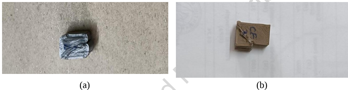
Figure 4: compression test specimens (ASTM D695) (a) silver nanoparticles induced PLA (b) copper nanoparticles induced PLA
