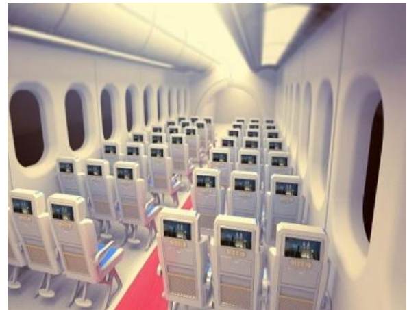
Figure 8 CAD illustration of the optimized passenger cabin design based on the fuzzy logic results
