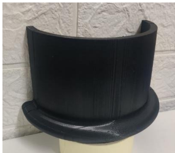
Figure 8 Scaled down A320 wheel model for curved surface scanning test
