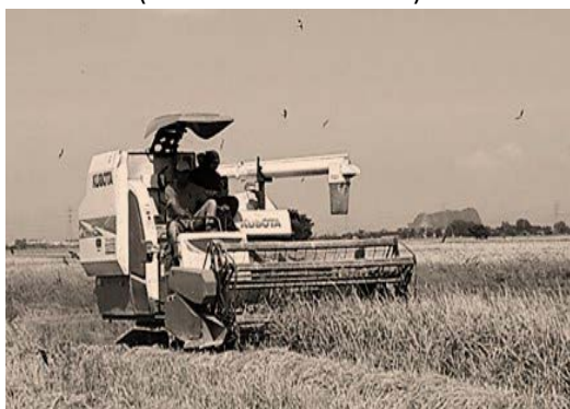
Figure 9. Typical medium combine harvester (Kubota model DC-95M)
