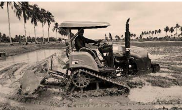
Figure 14. Triangular rubber tracked tractor attached with a rotary tiller
