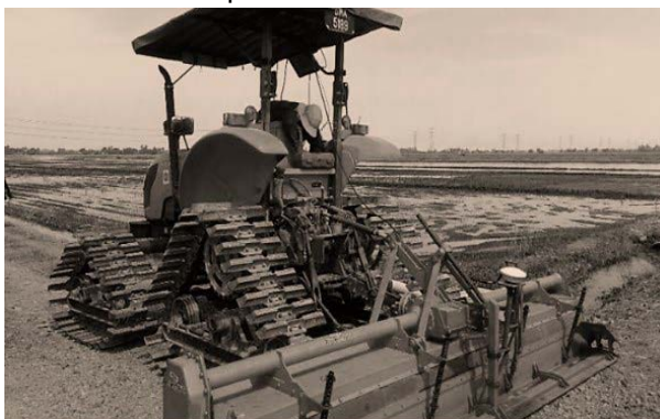
Figure 5. Automated land-leveling system mounted on a quad-steel-tracked tractor
