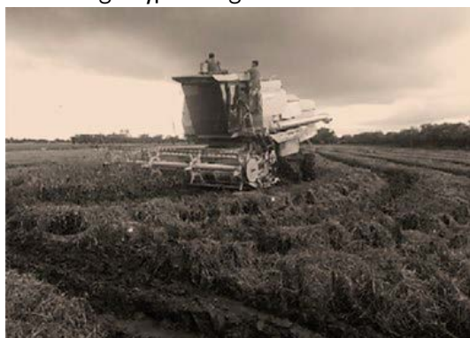
Figure 10. Paddy harvesting using a typical large combine harvester
