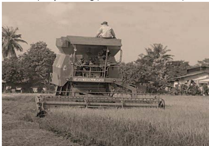
Figure 4. Typical large combine harvester used in paddy harvesting (New Holland model 1545)
