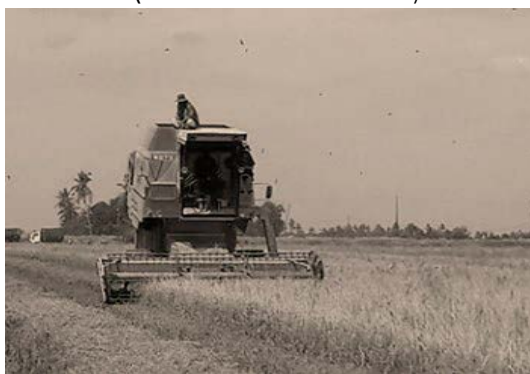
Figure 8. Typical large combine harvester (New Holland model 8070)
