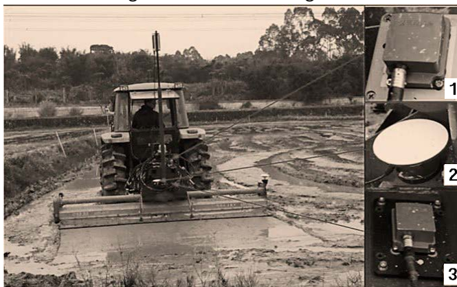
Figure 15. Land leveling operation using laser-controlled leveling-beater
