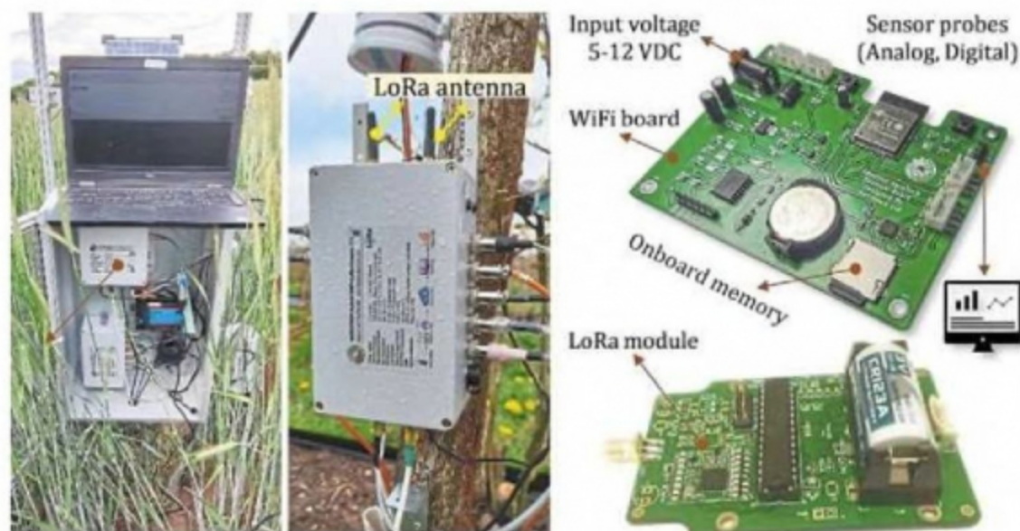
A multi-parametric sensing platform with IoT (Internet of Things) capability. – Adaptive AgroTech International
