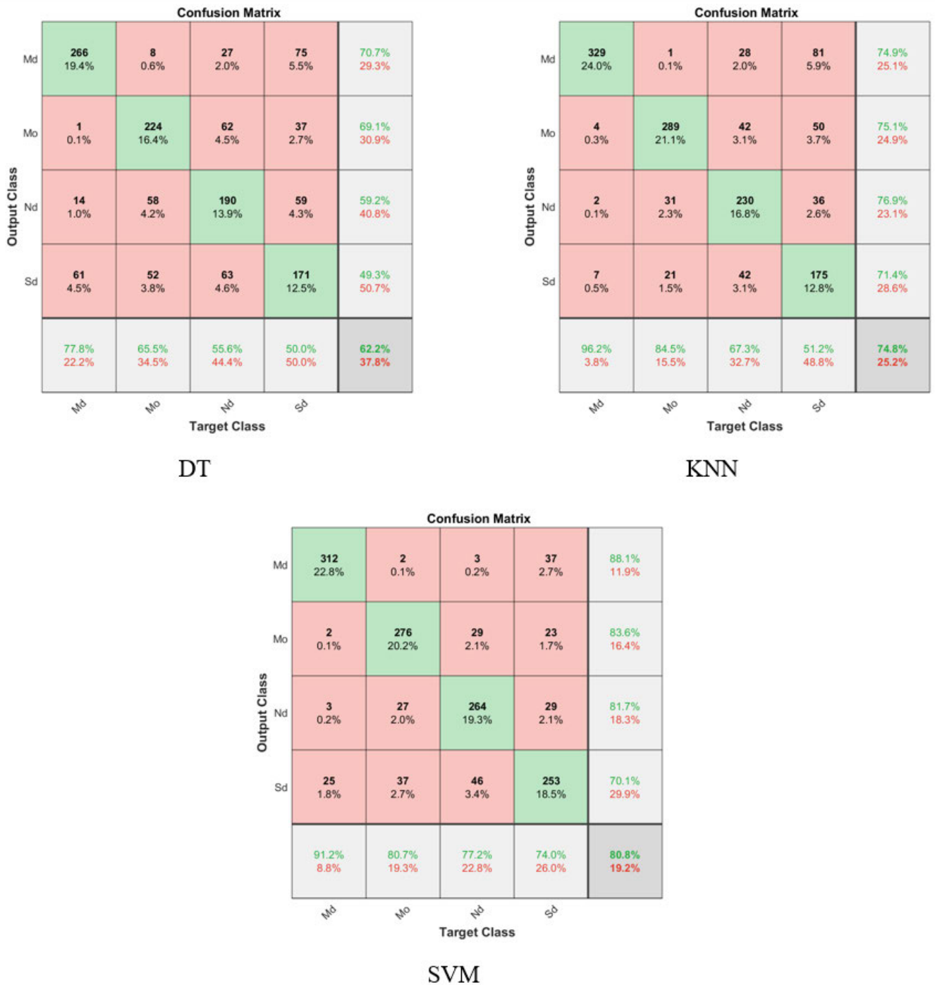
FIGURE 7. Confusion matrices utilising pre-trained MobileNetV2 with DT, KNN, and SVM classifiers for mild, moderate, and severe patients, together with normal subjects.
