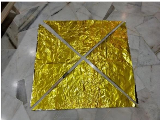
Figure 12 Aluminized Kapton Sail Membrane
