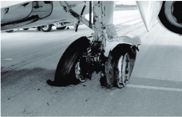
Figure 1 Possible aircraft wheel damage during landing phase [9]
