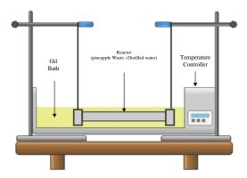
Figure 1. Subcritical water pre-treatment setup
