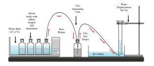
Figure 2. Anaerobic digestion set-up
