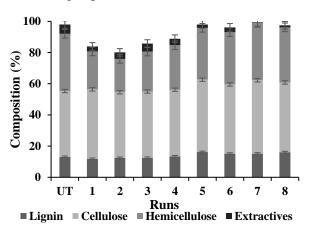
Figure 5 Pre- and post-subcritical water pretreatment compositional characterization.
