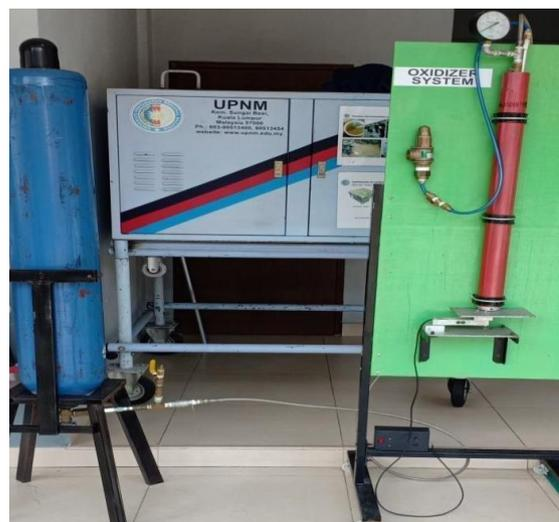
Figure 8 Oxidizer system test rig
