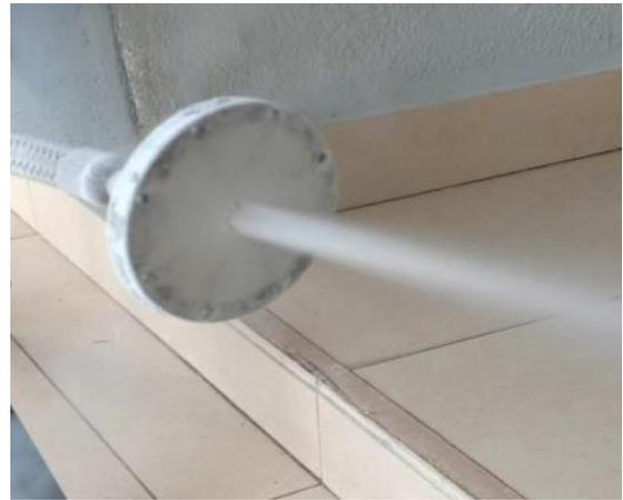
Figure 10 Oxidizer injector test
