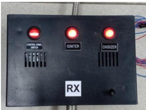
Figure 7 Radio frequency receiver unit
