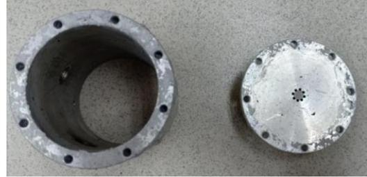
Figure 9 Bulkhead with oxidizer injector
