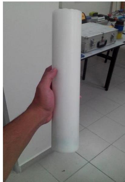
Figure 5 Fuel grain for the hybrid rocket engine
