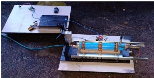
Figure 4 Static test stand for hybrid rocket engine
