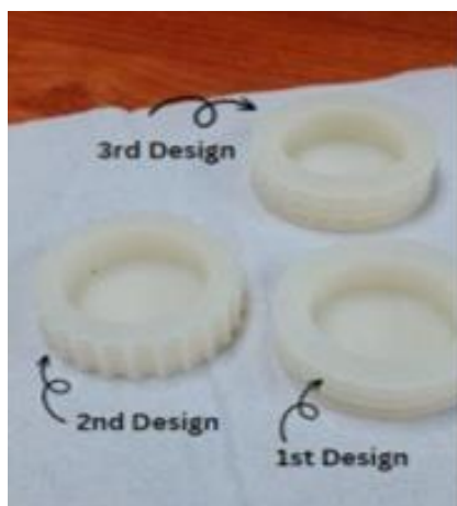
Figure 6 3D printed parts of modified Tesla turbines
