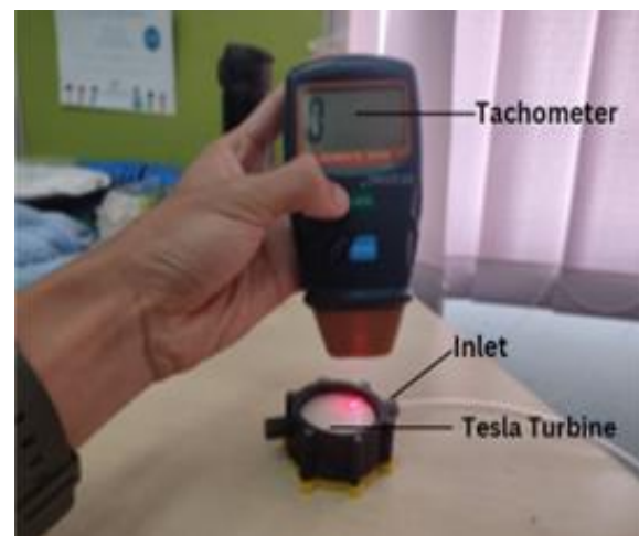
Figure 7 Measuring the RPM of the Tesla turbine.
