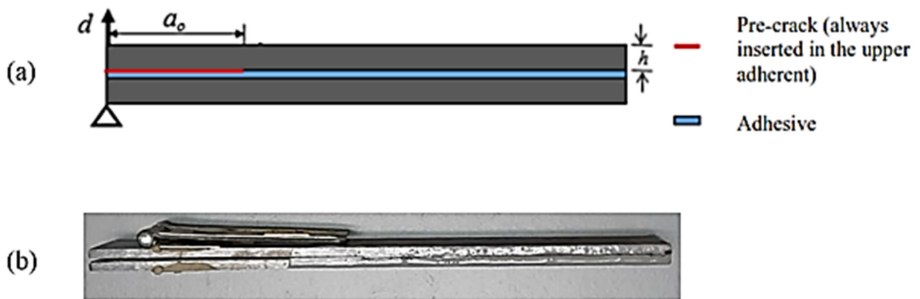
Figure 3. (a) DCB schematic representation; (b) the actual DCB specimen.
