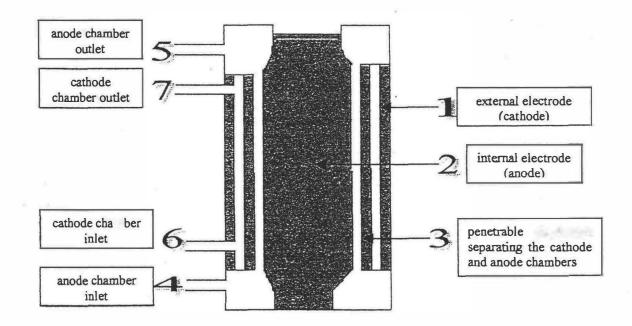
Figure 1.1: Flow-through Electrochemical Modular, FEM<sup>13</sup>
