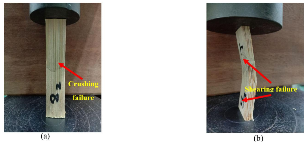
Figure 10. Failure mode of strips from four bamboo species for compression parallel to the grain: (a) failure due to crushing, (b) shearing failure in the bamboo strip.
