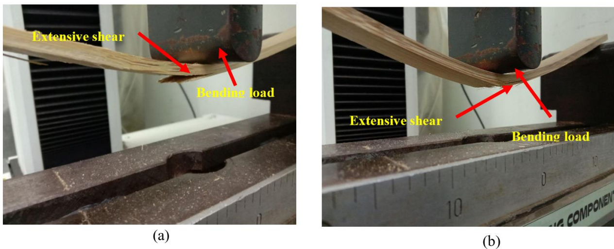
Figure 9. Failure mode of strips from four bamboo species loaded in static bending: (a) brittle shear tension mode, (b) splintering tension mode.
