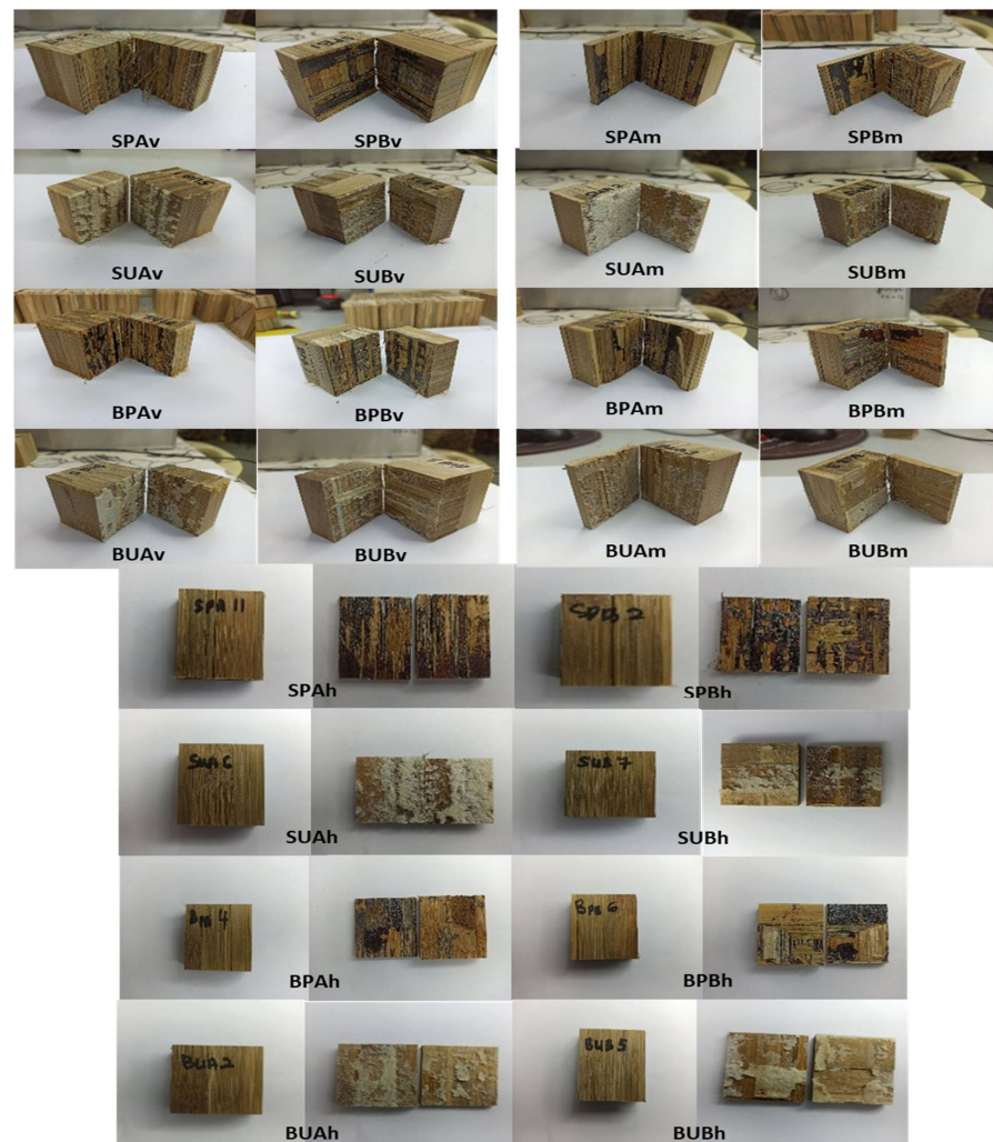
Figure 7. Sheared samples of laminated bamboo boards fabricated with different species, adhesives and configurations. Note: SPA—Semantan PRF parallel; SPB—Semantan PRF perpendicular/cross; SUA—Semantan PUR parallel; SUB—Semantan PUR perpendicular/cross; BPA—Beting PRF parallel; BPB—Beting PRF perpendicular/cross; BUA—Beting PUR parallel; BUB—Beting PUR perpendicular/cross; v—vertical arrangement; h—horizontal arrangement; m—mixed arrangement.
