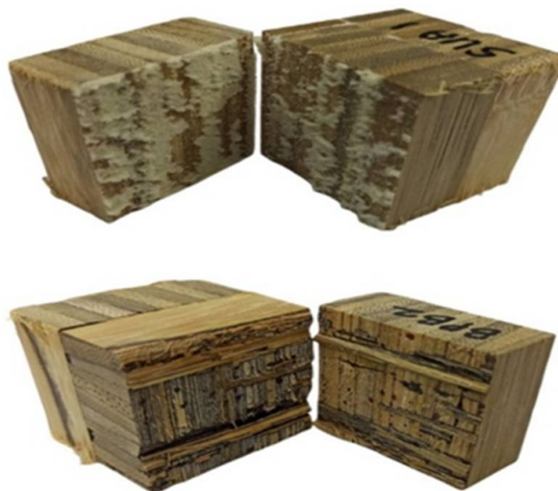
Figure 4. Sheared samples for failure estimation after shear test.
