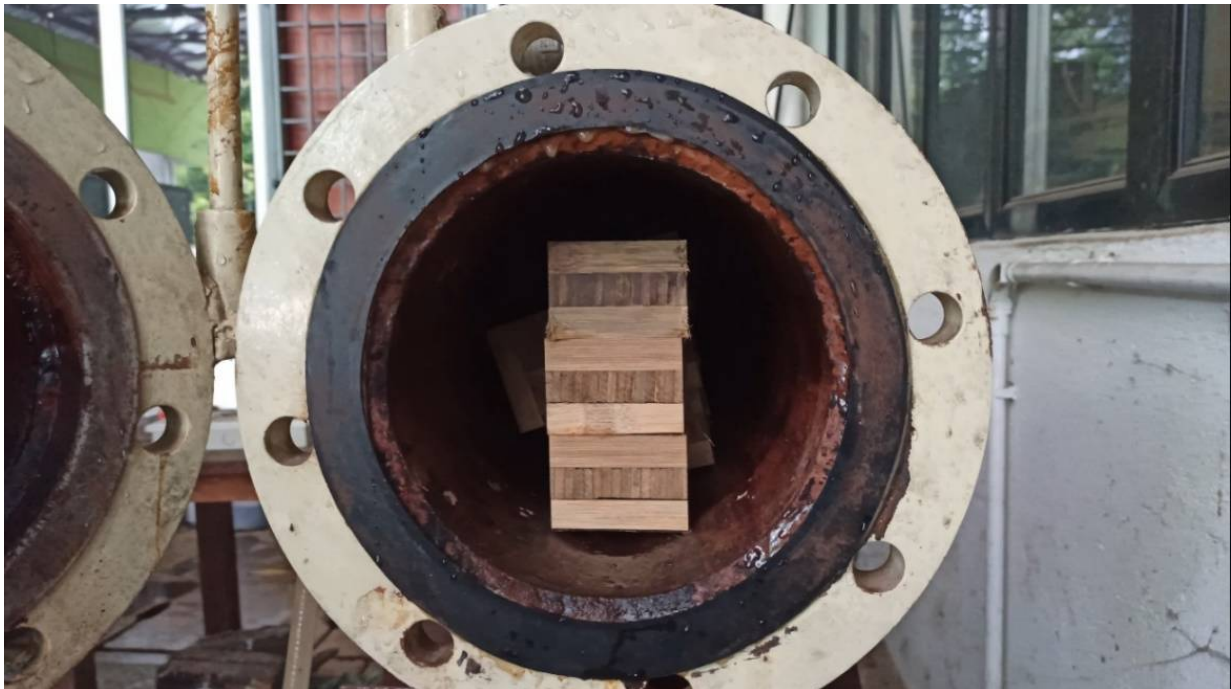
Figure 5. Samples placed inside a pressure vessel for delamination tests.
