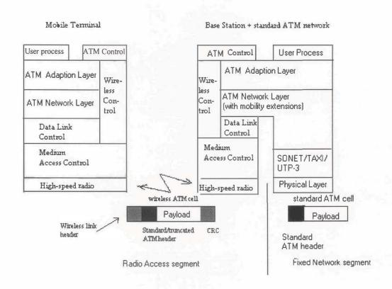
Figure 1. Wireless ATM protocol stack
