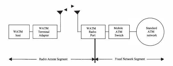
Figure 2. Wireless ATM reference architecture
