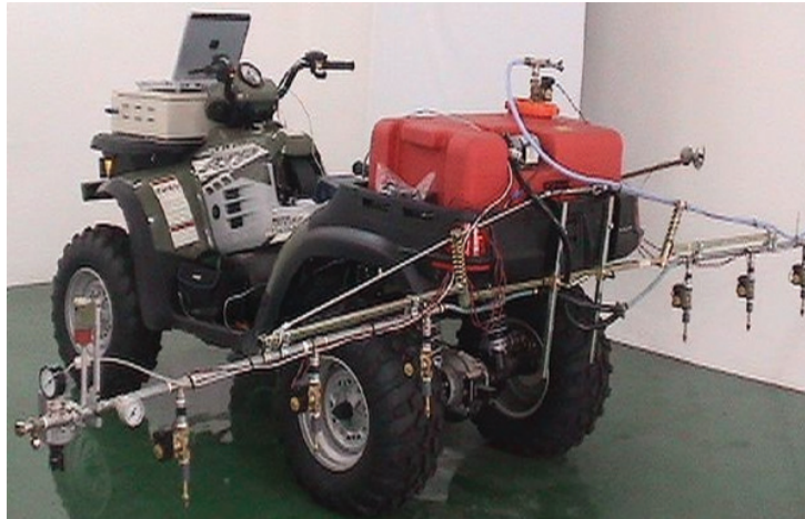
Fig. 1: A web camera and communication devices installed to the automatic sprayer
