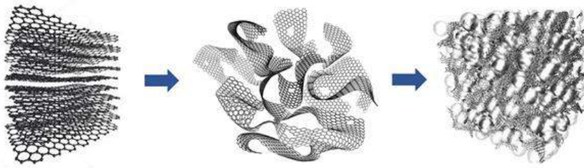
Figure 1.1: Illustration diagram to construct 3D graphene from graphene layers. The construction of graphene in 3D mode can allow the full utilisation of surface area due to suppressed restacking of the sheets. (Image taken from Hiew et al., 2018)
