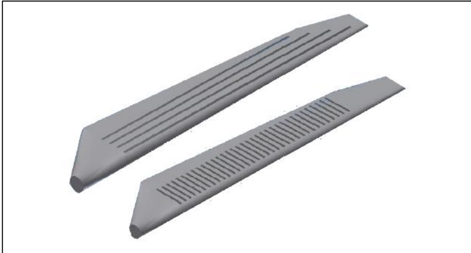
Figure 2.2: Unconventional design propeller of slotted propeller (Kutty & Rajendran, 2017)
