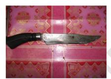
Figure 1.3 : Knife used to dehusk the mesocarp of palm fruitlets
