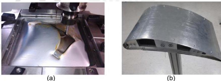
**Figure 1.2 : Example of automotive and aerospace components manufactured by ISF (a) car fender and (b) airfoil**
