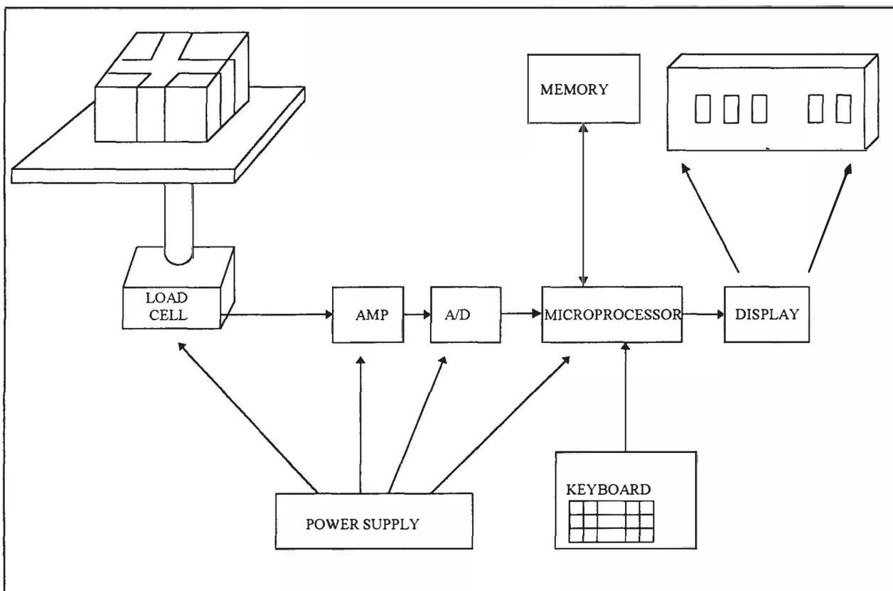
Figure 2: Block diagram of microcomputer-based smart scale
