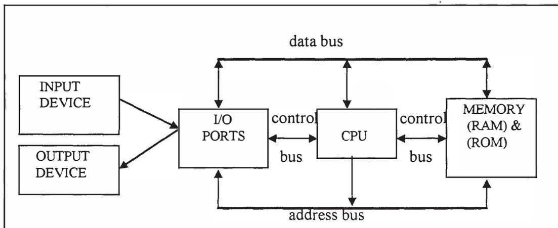
Figure 1: Block diagram of a simple microcomputer
