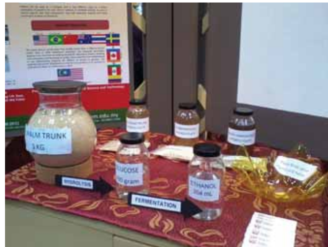
Figure 1: A display that shows the optimum bioconversion process of lignocellulosic waste to ethanol
