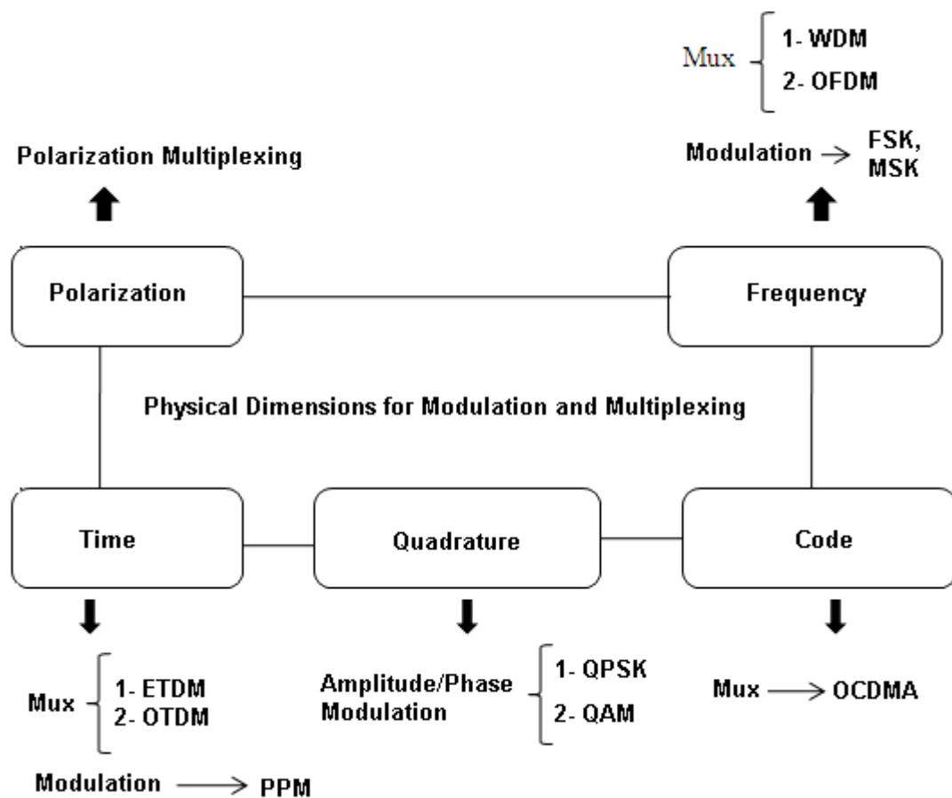
Figure 1-2: Physical dimensions that can be used for modulation and multiplexing in optical communications [2, 6, 7, 23-25].
