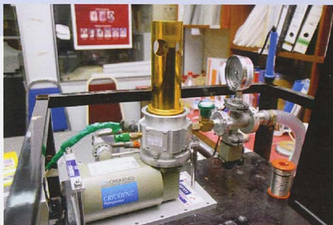
The overall set-up of the cooling chamber for the four-point resistance measurement system.
