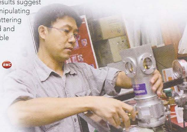
This is the electrical system for determination of superconducting transition temperature.
